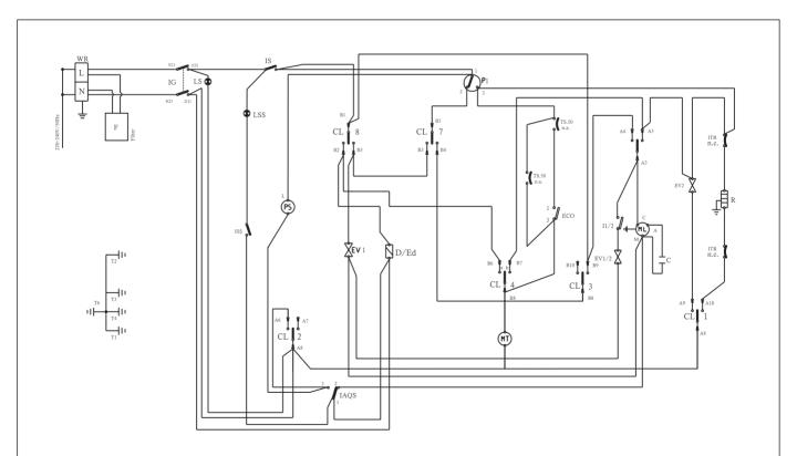
WR: Wiring box IG: Power switch IS: Door switch P1: Water level switch LS: Power indicator LSS: Salt missing switch ISS: Softener switch PS: Drain pump EV1: Inlet valve D/ED: Dispenser ECO: Economic wash switch TS58:58°C temperature controller TS50: 50°C temperature controller ITR: Temperature limiter R: Heater EV2: Softener valve ML: Washing motor MT: Timer motor IAQS: Overflow switch I1/2:Half load switch EV1/2:Half load valve
